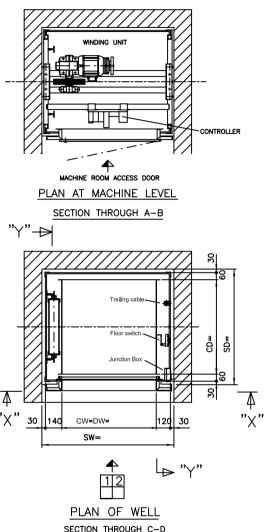
NOTE! LIFT CAN NOT BE INSTALLED UNLESS ENTRANCE WALL IS LEFT FULLY OUT!
