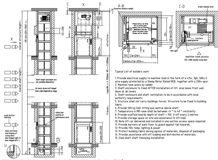
Ceiling below the lift shaft must support all strengths from the lift and must be calculated with a minimum of 5 kN/m<sup>2</sup>.
